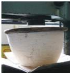
Figure 8. Test of Strength Vetiver Waste Pot
