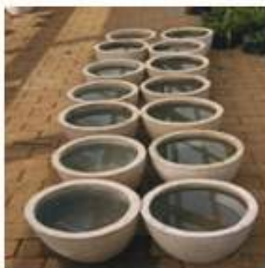
Figure 7. The Seepage Test of Waste Vetiver Pot
